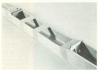
Row 1: (L) The tail fin has a soft core and alternating grain to save weight and increase strength. (R) Tail boom is pre-shaped before fitting tail fin in place. Note extended tail fin core keys into tail boom.
