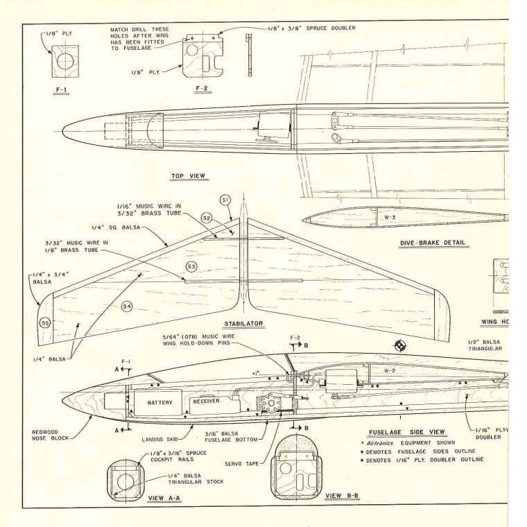
the leading edge center section of the wing to fit the fuselage saddle, leaving 1/16" clearance at F-2.
