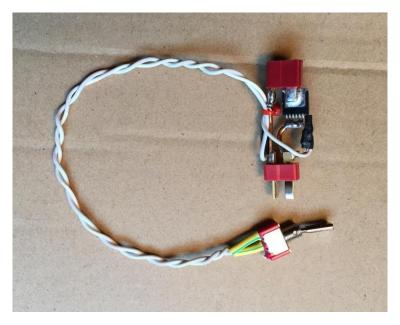
Insulation and a strain relief tie have been added.
