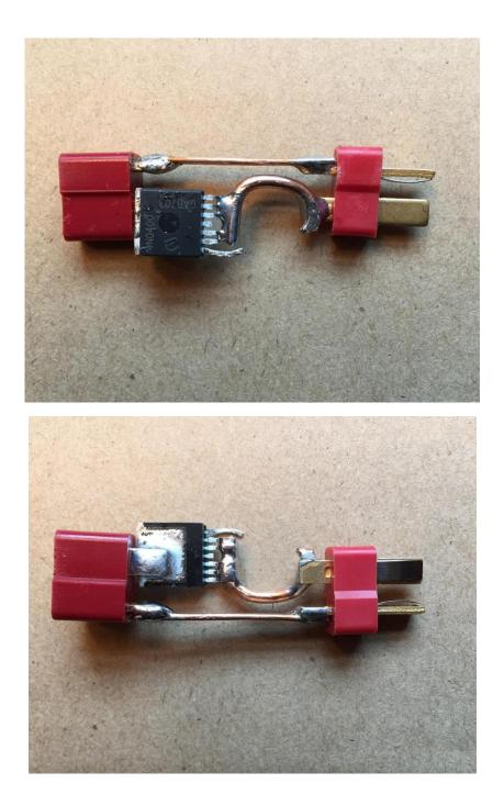
The power handling components. Top view and bottom view. The #12 awg copper conductors are stripped from 20A household wiring. Some of the conductors have been hammered into flat ribbons to better fit the connector terminals. You can see the gate terminal lifted up from the MOSFET.
