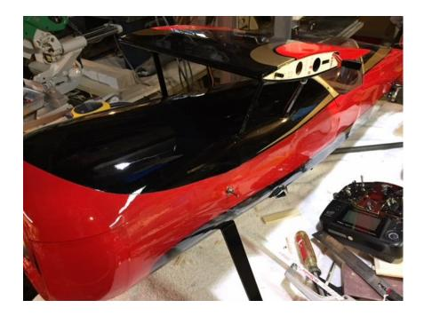
Tiny switch, big improvement in safety and performance! Mount the switch so that the model powers up when the switch is UP. Always have the switch OFF when installing a new battery.
