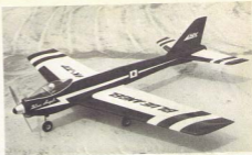
The latest version of the Blue Angel shows an even shorter nose, with a deeper profile to accommodate retract, the absence of any wing fences and a redrafted vertical tail.
