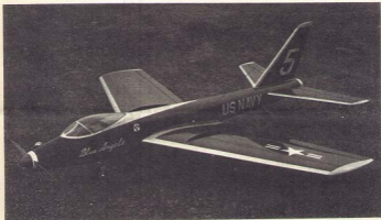
The prototype Blue Angel, as designed by Mr. Kato after he was influenced by the Navy's aerobatic team. Note the long nose and wing fences.
