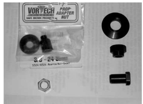
Home Depot 3/8-24 nut and Dave Brown spinner adapter washer on left, and heavy stock OS/ spinner adapter hardware on right
