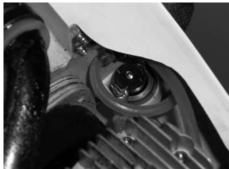
Top of Perry pump mounted to firewall
