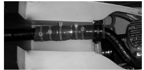
Two coupler stress relieving setup for Mueller header. Also note placement of one spring clamp
