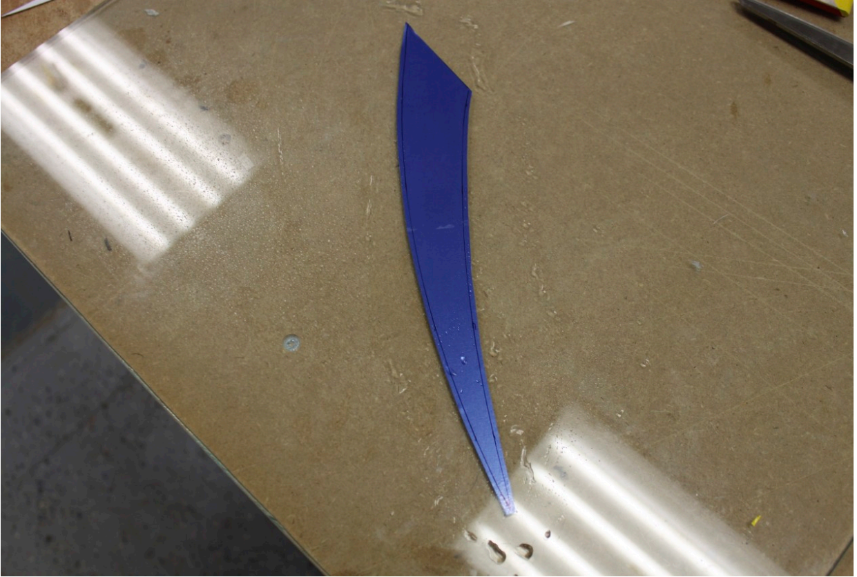
Now iron the blue in place using some guides to keep it aligned.
