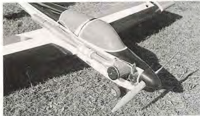
In both AMA and FAI applications, a Webra .61 Long Stroke was the power choice complemented by a Macs Products tuned pipe and 11 1/4-10 1/4 Yoshioko prop. Fuel used was S&W 7%. Output was 11,300 RPM.
