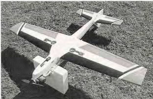
The wing attaches with four 1/4-20 nylon bolts through hardwood bearing dowels drilled into the wing (above). The tail end gets a little "busy" with pull-pull rudder cables and dual elevator pushrods exiting the rear. Equipment installation in the fuselage (below) needs careful consideration. The two forward servos handle the nose gear retract and throttle; the two rear servos are elevator and rudder/steering.
