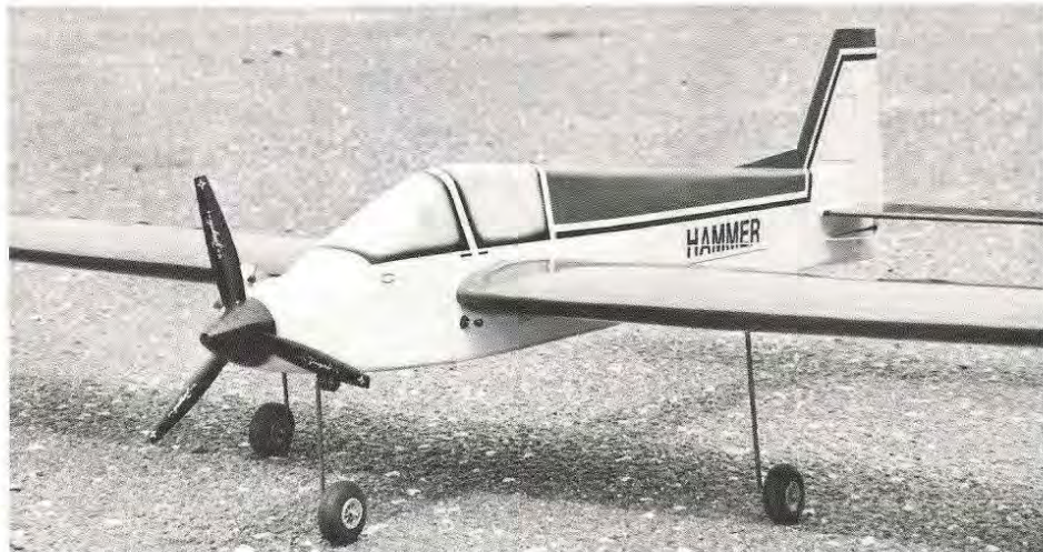
Dick's mid-wing version used the latest version of the K&B .40 with a 3-bladed Zingali prop and a Mac's Products muffled tuned pipe.
