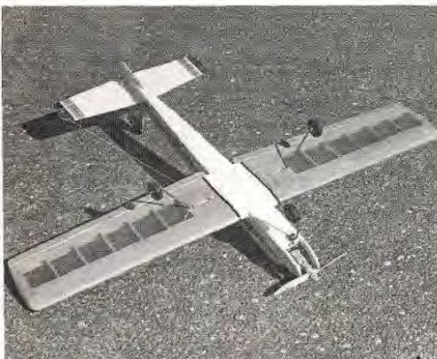
You won't see the Pepper in this position much (we hope). Purpose of this bottom view reveals the conventional tricycle gear arrangement.
