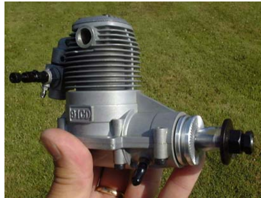
RCV91CD is the same physical height as a typical 48/52 conventional 4-stroke
