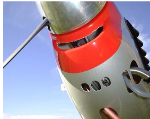
Mustang cowl has additional outlets for cooling air – as a general rule outlets should be three times the area of inlet holes
