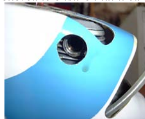
Mustang cowl has additional outlets for cooling air – as a general rule outlets should be three times the area of inlet holes
