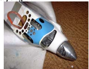
Mustang cowl has additional outlets for cooling air – as a general rule outlets should be three times the area of inlet holes
