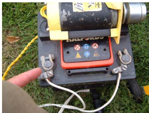
If starting from behind the propeller, remember to reverse the leads!!
