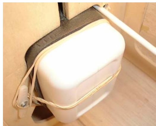
16 oz tank in Hangar 9 Mustang gives more than adequate duration for its RCV 91 CD
