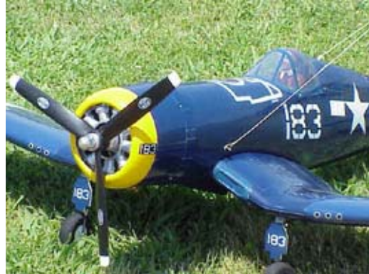
16x10 3-bladed prop on RCV60SP
