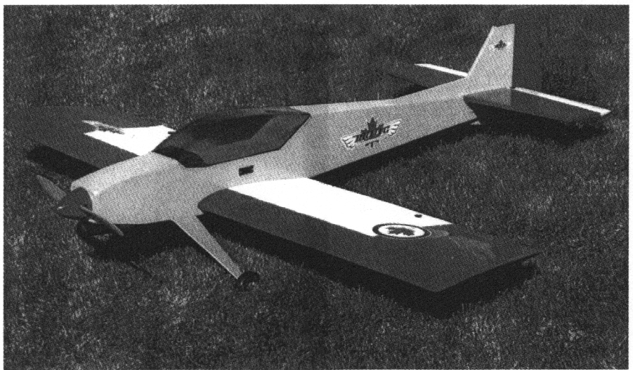
Finished airplane showing clipped wing, modified tail surfaces (above). Lots of easily seen color changes—bright red and white wings, bright yellow body. Side mounted engine (below) for proper fuel flow during maneuvers and lots of cooling air past the engine head.
