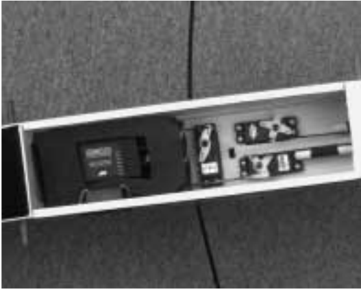
Fuselage Servo, Receiver, Battery Installation
