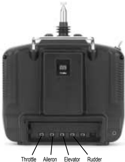
Servo Reversing Switches (Located behind Transmitter Battery Pack)
