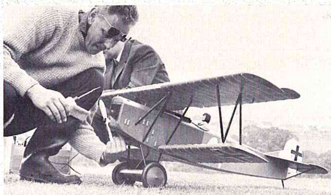
Opening the needle valve prior to starting.
