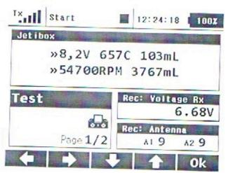
In case that you would like to select another sensor via the Jeti Box Function, you have to leave the JJXC via ECU Menu by pushing the upwards arrow for some seconds. It is then guaranteed that the alarm signal is further displayed (Morse code 'M' and 'U').
