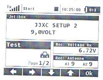
Via Jeti Box the Voltage Alarm is displayed with the Morse code 'U'. Please push the "Arrow downwards button "at the Jeti Box transmitter controller again. The adjusted Voltage Threshold gets saved in JIXC. In the following the regular CB Electronics welcome page is displayed. From this page you can change tot he normal ECU Display Page.
