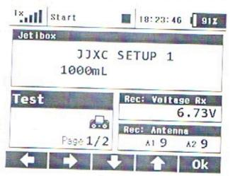
Please push the 'Arrow downwards button 'at the Jeti Box transmitter controller. The adjusted Kerosine threshold gets saved in JJXC. In the following the Setup Position-2 Voltage Alarm is displayed.
