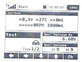
In the upper row you see the ECU operating voltage, the exhaust temperature EGT and the fuel flowrate of the Kerosine pump. In the lower row the turbine driving-speed and the tank volume is displayed.
