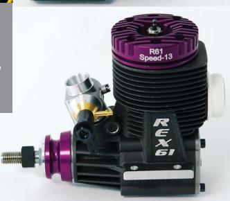
The single-piece crankshaft is machined from bar stock steel, hardened and finish-ground on all bearing surfaces. The asymmetric counterbalance adopts Novarossi's new turbo flow design concept aimed at maximizing the air/fuel mixture intake. This is the first time I have seen such a forward-thinking asymmetric crankshaft design in a classic pattern engine. Two high-quality stainless steel ball bearings support the crankshaft. The counterbalance design exposes a fair
