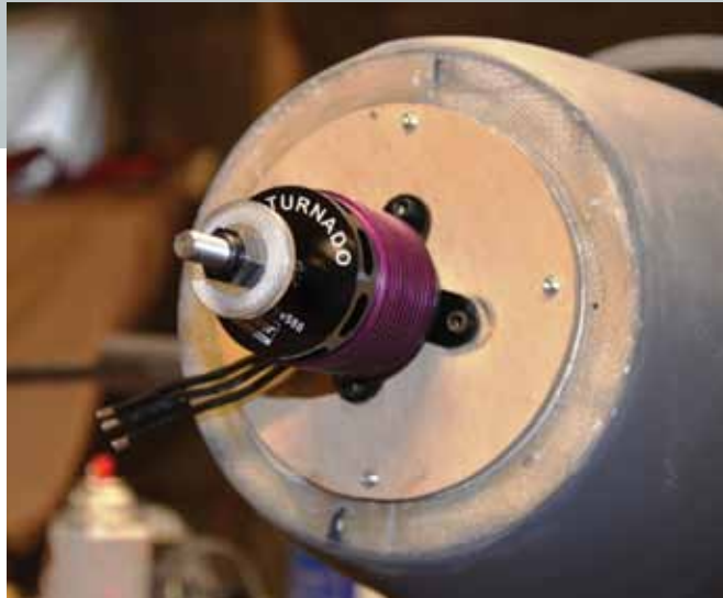
Here you see the Hacker A50-10L Turnado bolted to the Komet's firewall. It is an excellent choice for this WW II flying wing design.
