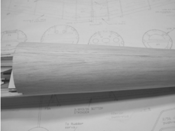
4. Using laser-cut 1/16 balsa, sheet front bottom. Sheet from main stringer to hatch rail (leaving half of hatch rail un-sheeted for hatch installation).
