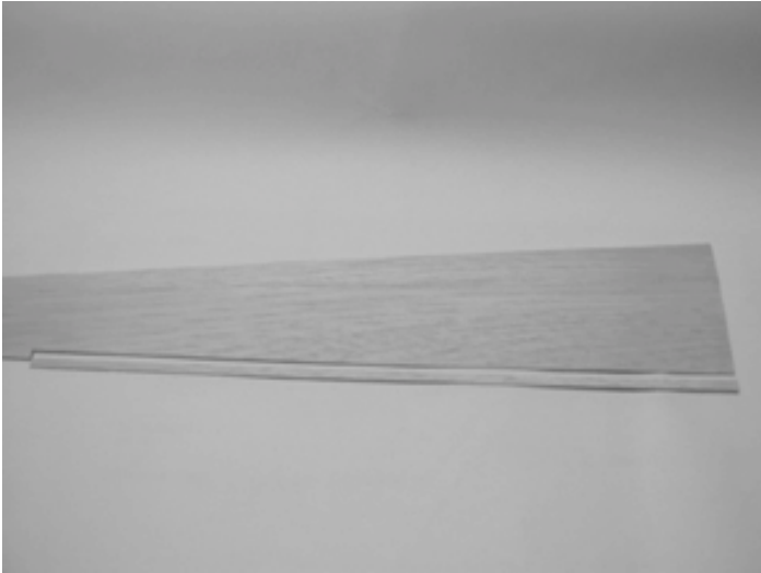
2. Pin made sheet to main spar and bend it toward the rear bottom stringer. Mark center of the bottom stringer on the sheet. Cut as marked and glue sheet in place. Starting at main stringer and going to bottom stringer.
