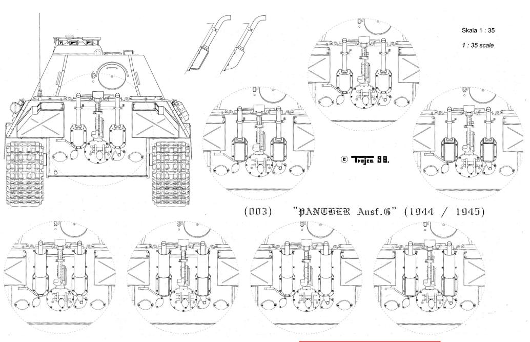
Single exhaust pipe with horizontal brackets (cast armored covering on left, welded on right)
