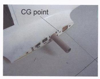
**5 lbs. lead in nose** on bottom LG tray...3 batteries in top tray...measures about 1.25 lbs nose heavy at cg hole. This model likes to be a little nose heavy... balanced at cg hole created slight tail heavy feel...takes LOTS of down trim to control.... Exact balance at cg hole also causes plane will jump off at takeoff and possible kangaroo at landing
