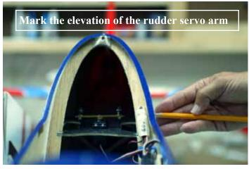
holes on the control horn on the rudder need to be 2 inches from hole to hole if you use that servo arm.
