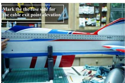
Start by temporarily installing the rudder with the control horn installed. Install the rudder servo with its control arm. Now you can mark a line on the outside of the fuse at the height of the servo arm (see photo 1). Just visually sight it and make the mark. Now, lay a long rigid straight edge on top of the control horn and through the line you just made on the fuse for the servo elevation. Mark the fuse along the straight edge near the rudder where the cable will exit. This line
