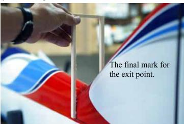
tool is 2". Using that tool, slide it over the rear fuse and mark where it just touches the fuse and the line that you drew using the straight edge. That mark is the exit point for the
