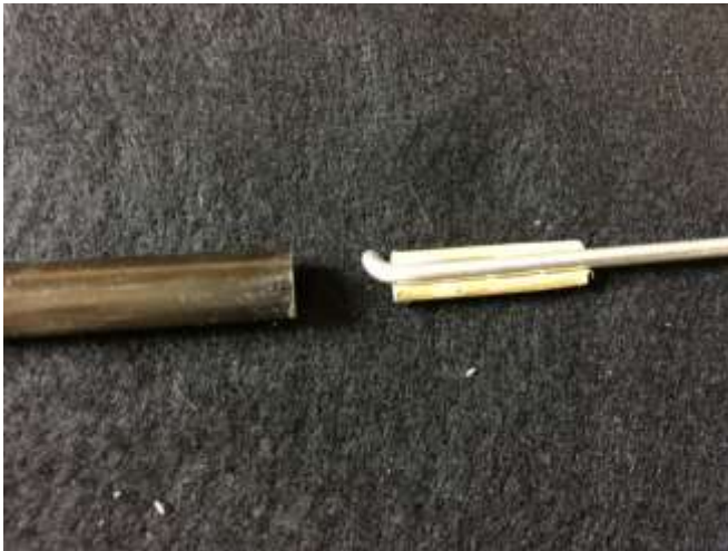
90 degree bend in pushrod shown.
