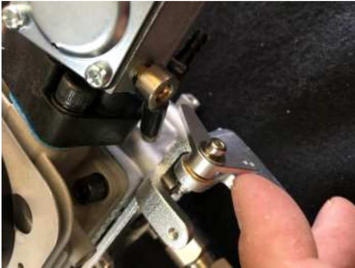
Carb bellcrank and carb arm in place. Optional 3558 aluminum arm shown.
