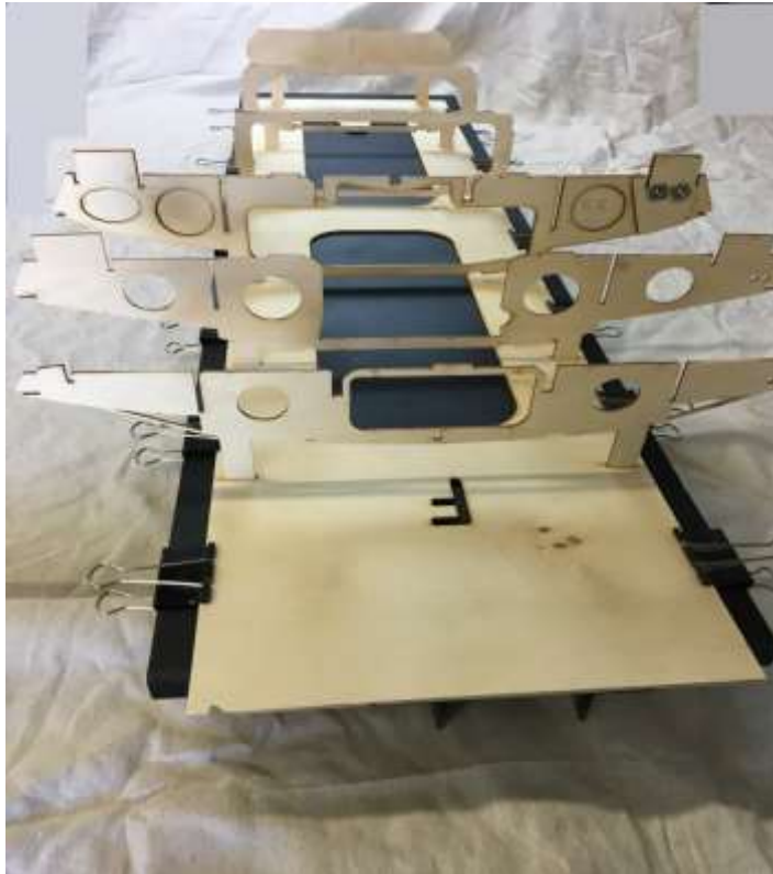
Our building board is two pieces of \frac{3}{4} MDF.
