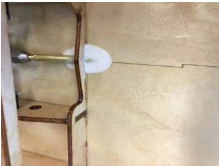
This stuffing tube will stay in place.
