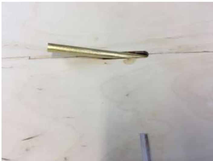
11/32 stuffing tube protruding from hull bottom.
