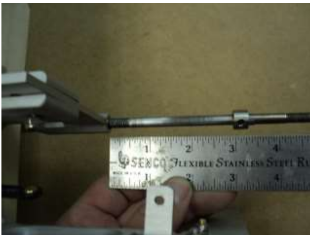
Measuring flex shaft for cutting.
