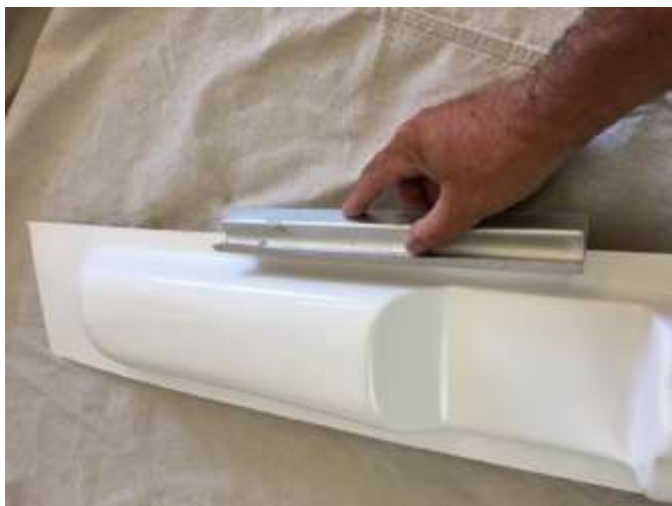
Sanding cowling edges. Sand well.
