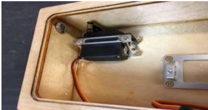
Throttle servo in position. Note EZ connector.
