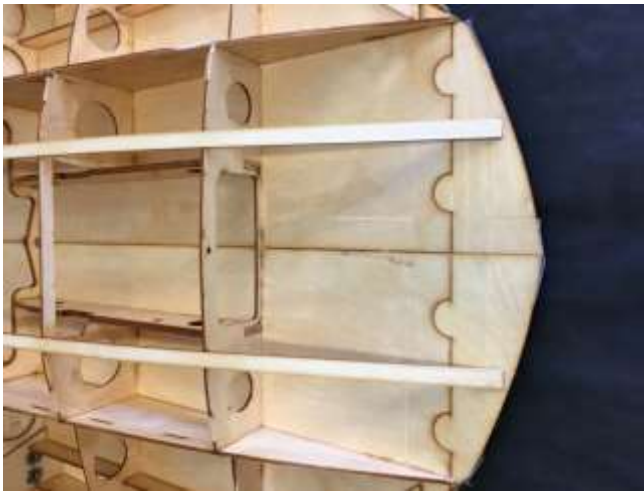
Cowl deck supports glued in place
