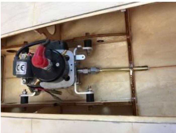
Engine rails are pre-drilled for Zipp 3409 mounts.
