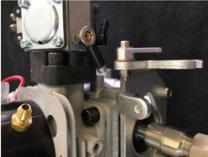
Bellcrank pushes arm open. Throttle spring closes.
