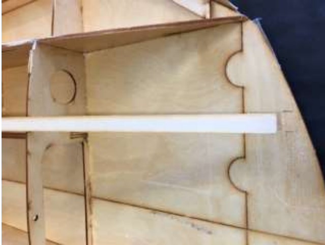
Cowl deck support parallel with side.
