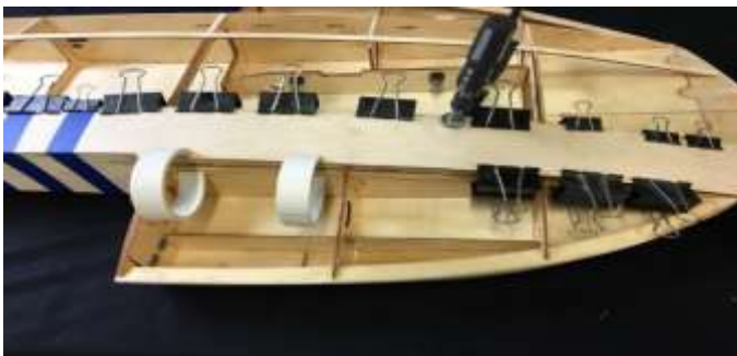
Deck being glued in place with epoxy.
