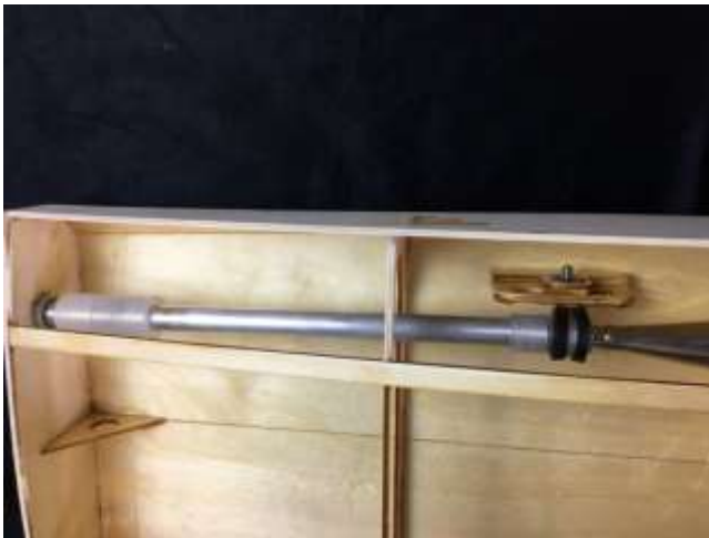
Pipe, extension and outlet. Use zip ties to secure.
