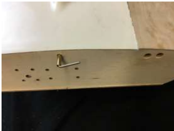
Latch pressed in. Don't glue until paint.
