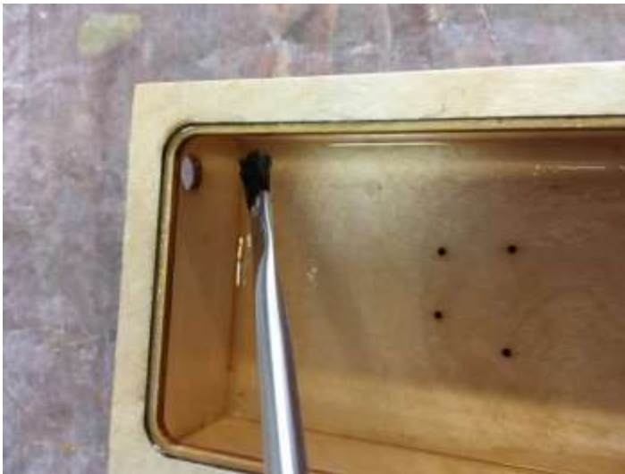
Sealing seams of radio box.
