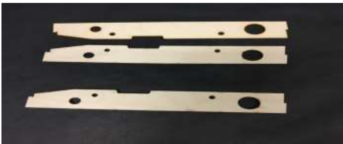
Engine rails before laminating (above), and after.
