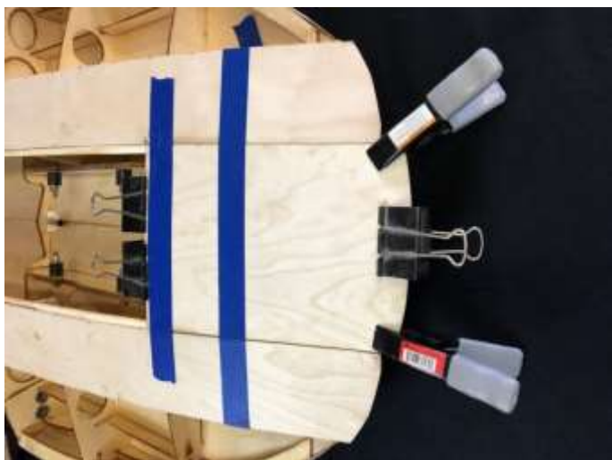
Deck center fitted and glued.
