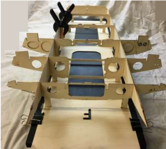
Side stringer being glued in place. Note clamps.
