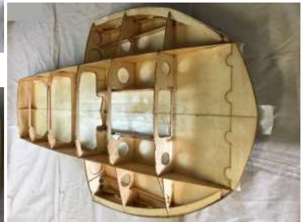
First coat of epoxy resin.
