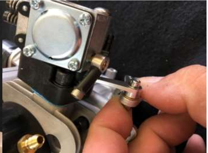
Carb bellcrank and carb arm in place. Optional 3558 aluminum arm shown.
