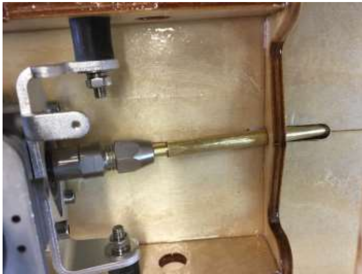
Using brass tubing to align the stuffing tube.
