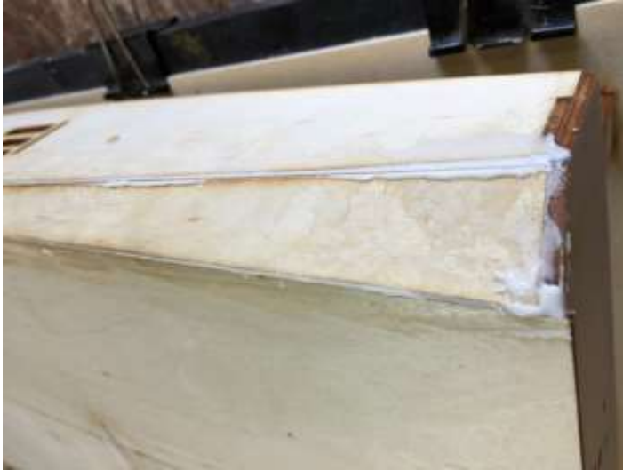
Epoxy/ micro balloons filler on rear non-trips.
