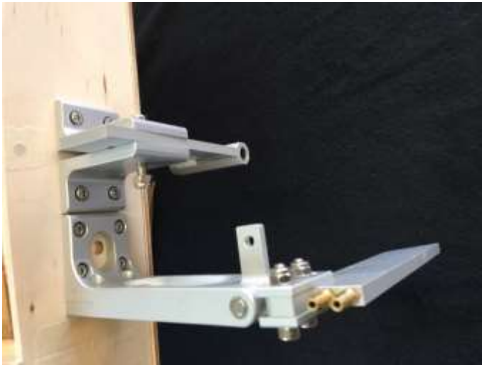
Strut and rudder mounted to transom.
