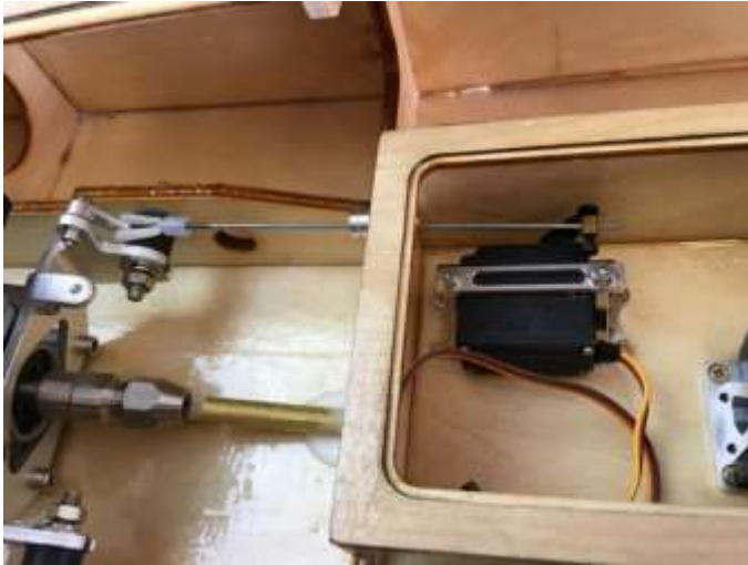
Throttle linkage. No carb in this picture.
