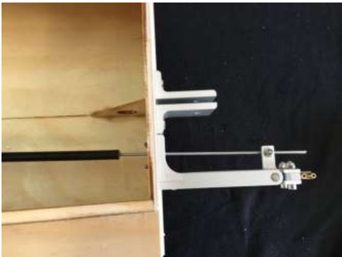
Rudder pushrod in place.
