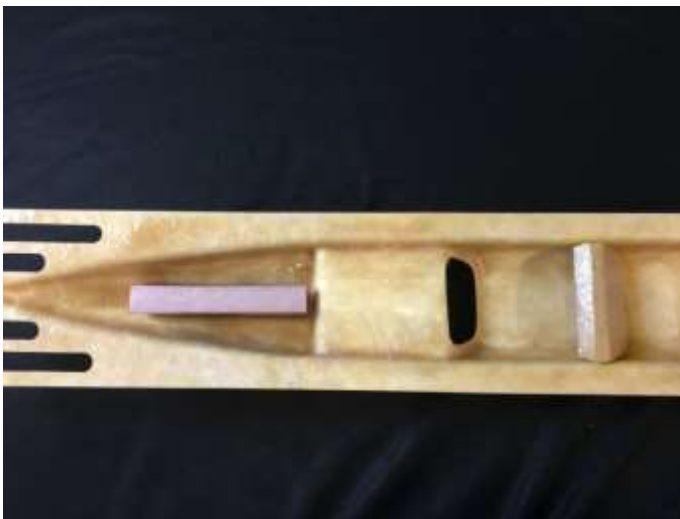
Foam floatation and air baffle in place.
