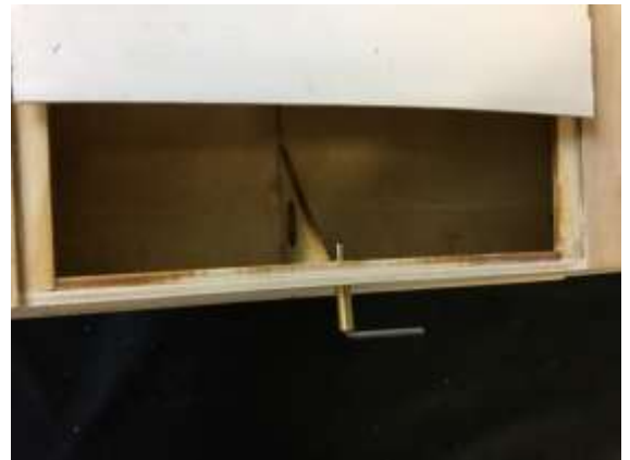
Latch installed, but not glued.
