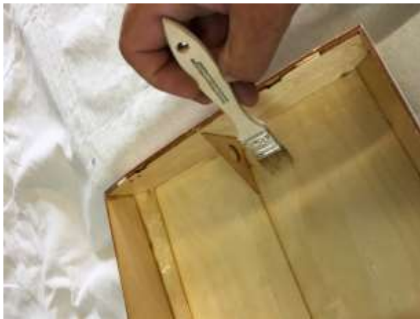
Second coat being applied after the first coat has fully cured.
