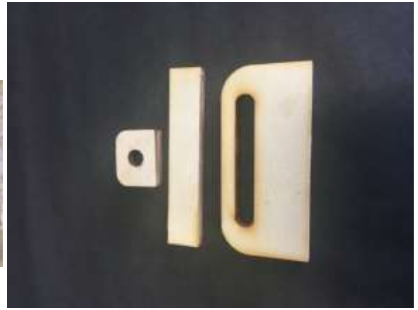
Pipe mount parts laminated.
