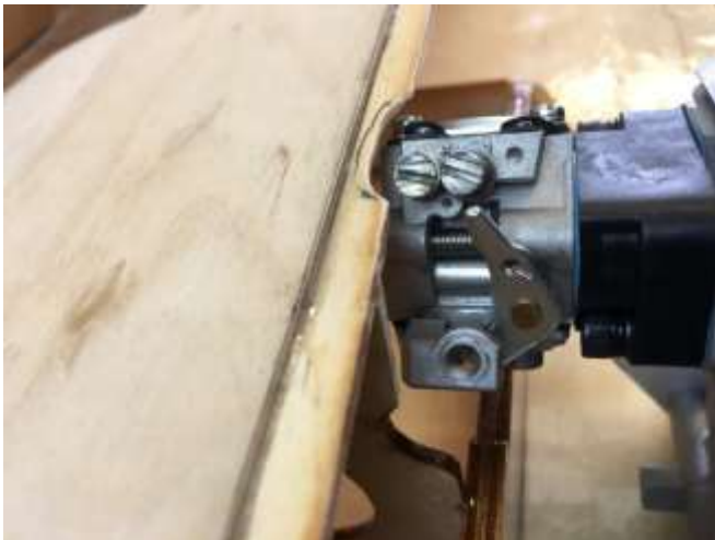
Deck support trimmed for carb clearance.
