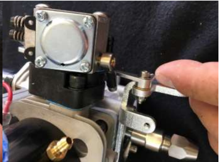
Carb bellcrank and carb arm in place. Optional 3558 aluminum arm shown.
