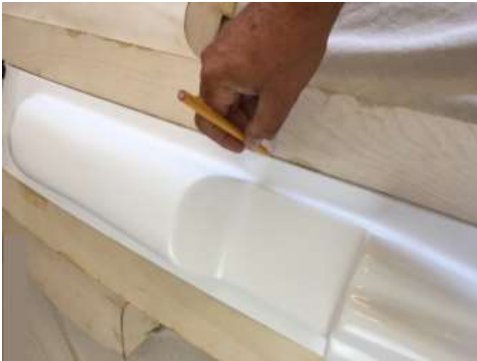
Marking decks for cowling.
