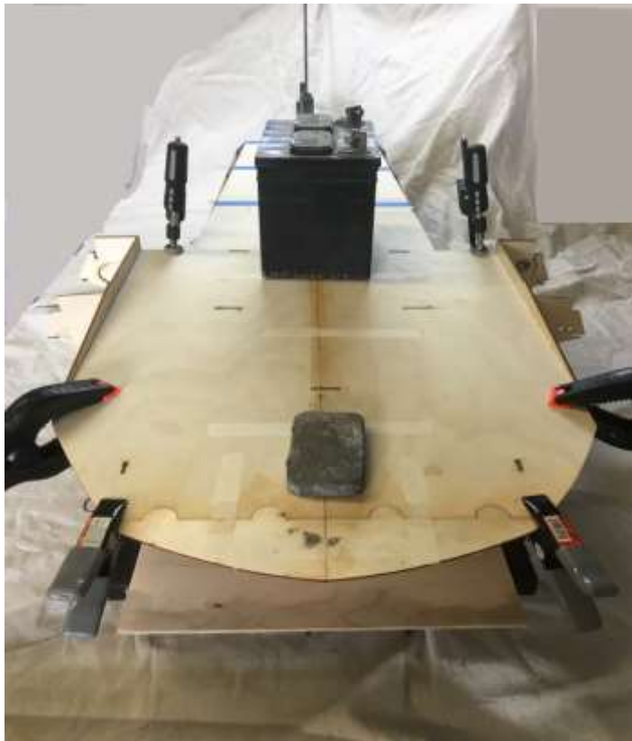
Lots of weight, tape and clamps on the bottom.
