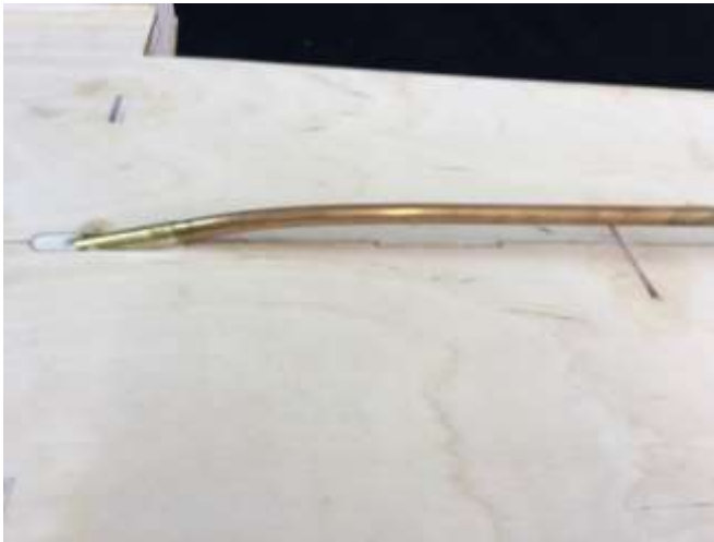
Shaft tube bent. Notice heat discoloration.
