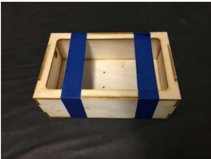
Tape radio box tightly while glue cures.
