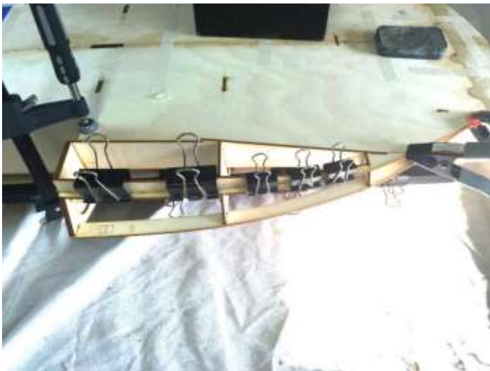
Spray rail glued in place. Clamp to SC.
