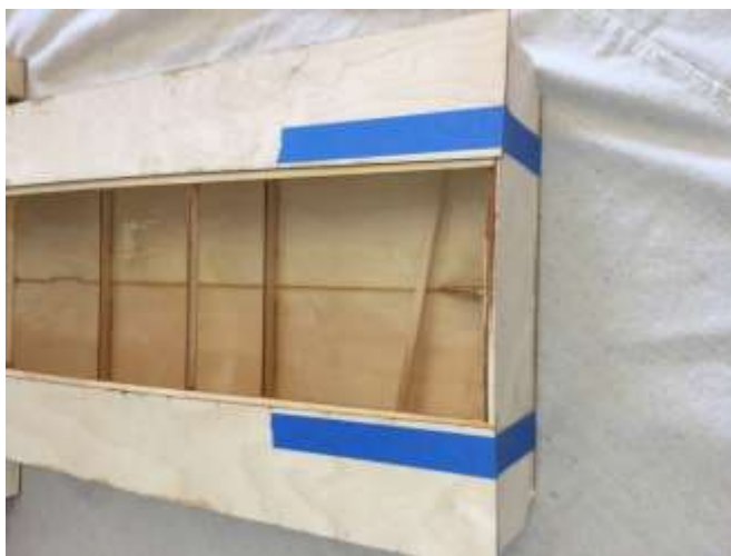
Top decks taped in place.
