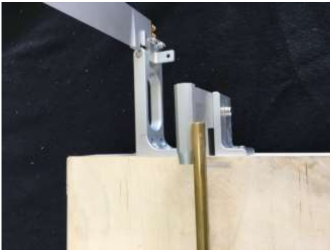
Shaft tube cut to fit into strut.
