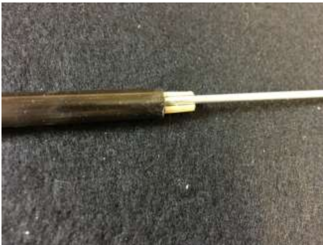
Epoxy everything into the carbon tube.
