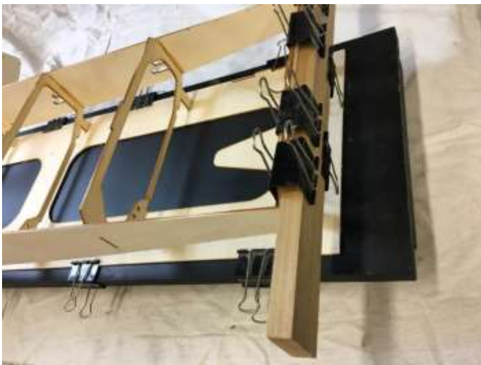
Wood clamped to transom to keep it straight.
