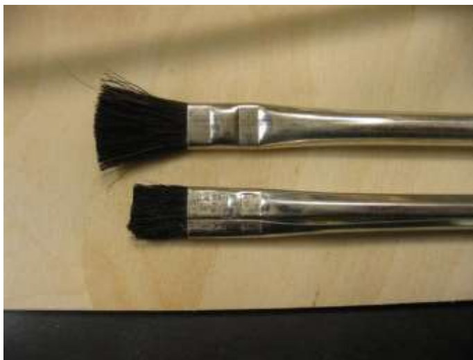
Epoxy brush trimmed for fast epoxy application
