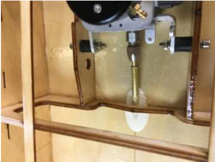
Epoxy with micro balloons makes a great filler.
