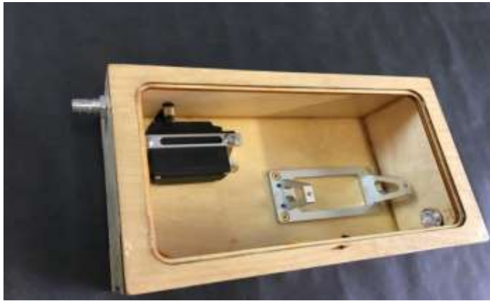
Servo mounts bolted to bottom.
