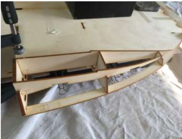
Sponson chine in place. Glue spray rail at the same time.
