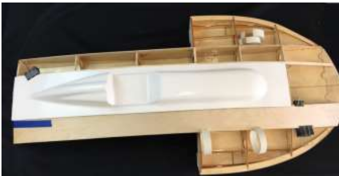
One deck in place being marked for trimming.
