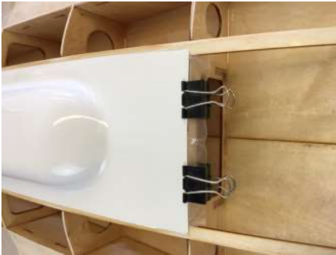
Gluing front cowl former.
