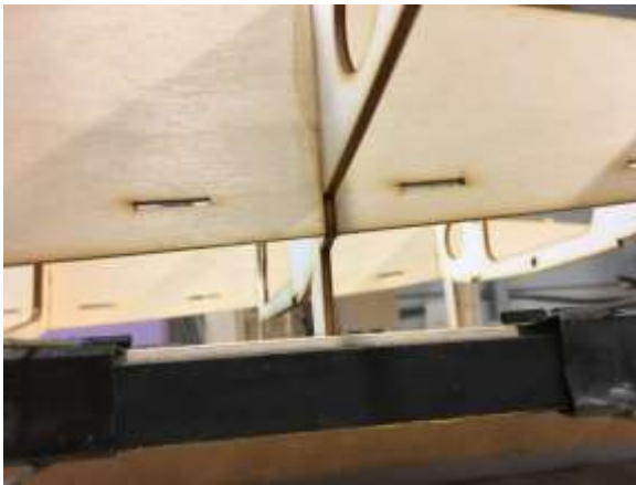
Side stringers flush with bulkhead edge.
