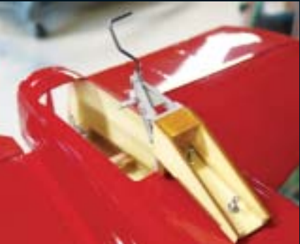
The Robart tailwheel bracket mounts to a plywood box that screws into the fuselage structure. I ran a pushrod forward to the servo to activate the retract mechanism.
