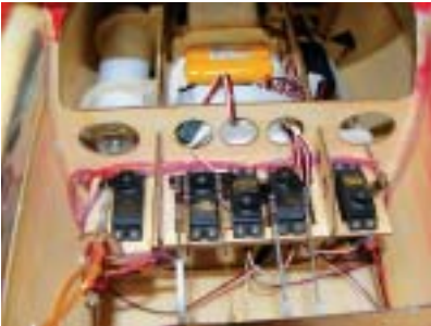
Looking forward in the cockpit. The servo tray is just behind the wing leading edge for easy linkage installation. The Robart air tanks, Futaba receiver, Duralite airborne battery with voltage regulator and fuel tank all mount forward closer to the firewall.
