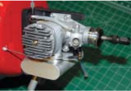
The O.S. 1.60 FX is plenty of power for the big Staggerwing. It can easily fly the model at partial throttle and wide open takes it upstairs in a hurry. Note the throttle pushrod took a little bend to reach around the muffler and get to the carburetor. The Bisson Pitts style muffler easily hides in the cowl.
