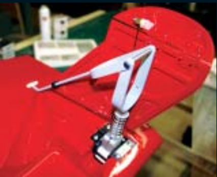
Top: The stock wire gear is designed to mount using the same bearer blocks as the more realistic Robart retract strut shown sitting in place. Above: The Robart gear with its rear strut installed looks like it came right out of the Beechcraft factory. Note the detail of the gear door, both inside and out.
