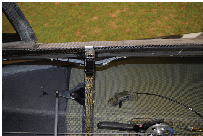
(Above) The retract 'handbrake' is on the RHS – the small lever outboard of it is the main undercarriage up-lock. (Photo: Brian Hope)
