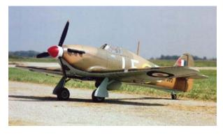
latex applied directly to the "raw" Coverite. The latex took to the Coverite like it was made especially for it. Great.... Nice thing here was that even when the fabric sags or takes a dent you can apply heat and re-shrink the fabric and the paint just goes along for the trip. Another thing I discovered is that latex paints don't crack due to vibration or expansion / shrinkage of parts. It's rubber, right....
