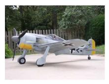
Hurricane also used this treatment). This works ok as long as the epoxy paint is not flooded on. You can't get the latex too wet with anything that has acetone or toluene in it. These chemicals turn the latex to a rubber cement kind of goo. On the second FW-190 I used latex for all the colors including all the camouflage and markings. The first FW-190 had a coat of satin clear epoxy over the latex, the second FW-190 had no clear coat on it. In my opinion the second one came out better.
