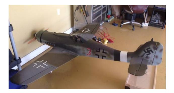
4. The wall is the DATUM reference for measuring. With the forward part of the plane (In this case the spinner) up against the wall, measure directly back from the wall to each axel center on the landing gear. Mains and tail/nose wheel.
