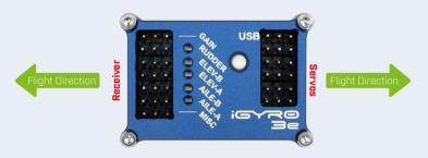
2. Connect the patch-leads to the receiver, and connect the servos.
