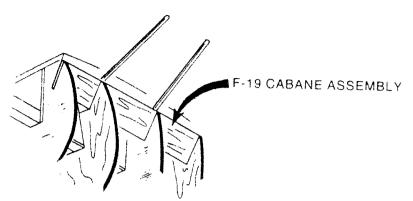
**NOTE:** THE FOLLOWING FUSELAGE SHEETING USED IN THE FOLLOWING STEPS RELATING TO THE GLUING OF THE FUSELAGE SHEETING TO THE FUSELAGE HAPPEN TO BE OVERSIZED, ALLOWING ONE TO TRIM AND OR FIT ACCORDING TO ONES EXPERTISE. REFERENCE TO THE POSITION OF THE SHEETING CAN BE FOUND ON THE TOP OF THE FUSELAGE PLANS.
