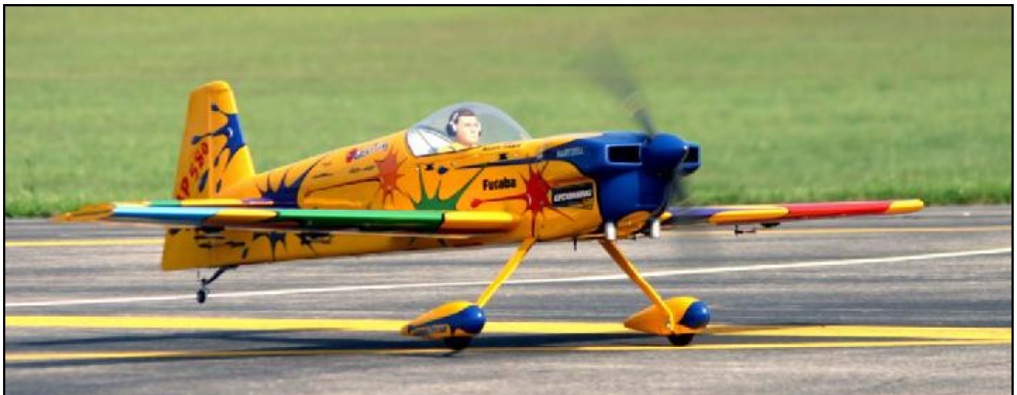
Mike Barbee flew in fun scale with his Great Planes CAP 580 1/3-scale ARF. A DA-100 engine powered the paint-splattered aerobat.
